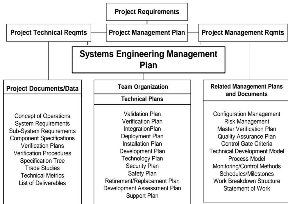
**Figure 12-5 Relationship of Systems Engineering Management Plan with Project Requirements**
