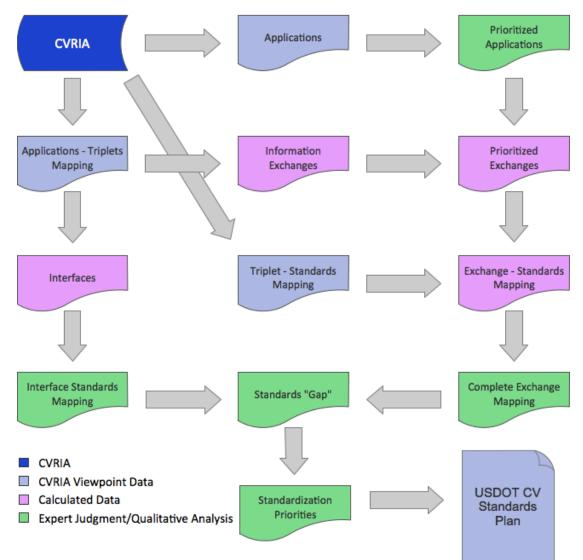
A "triplet" in the CVRIA is a combination of an information flow, its source, and its destination.
