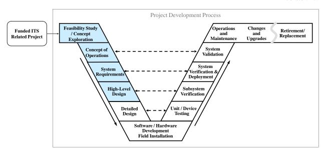
Figure 2: Use of Virginia NWR ITS Architecture in the Project Development Process
