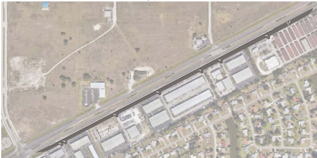
Conceptual Layout of Frontage Road (Continuous Right Turn Lane with Raised Barrier) SR 78, east of Andalusia Boulevard
