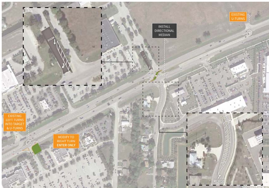
Conceptual Layout of RCUT at SR 78 and Hibiscus Drive
